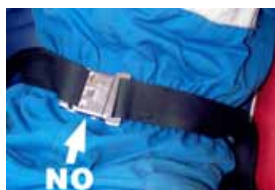
Incorrect position of the seat belt
